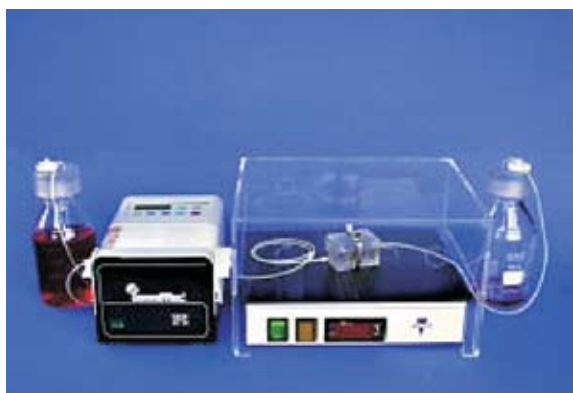
Minucell system used to develop the dynamic culture condition for Hybrid artificial lung model.
