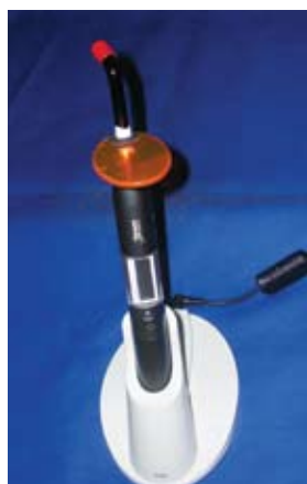
Novel dental light cure unit developed as per our request (410 nm wavelength)
